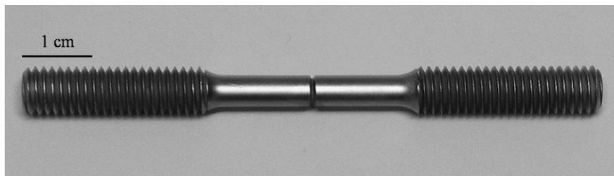
Fig. 1. A standard [10] tensile V-notch (TVN) sample made of AISI 4340 steel heat treated to 50–53 R<sub>C</sub>.
