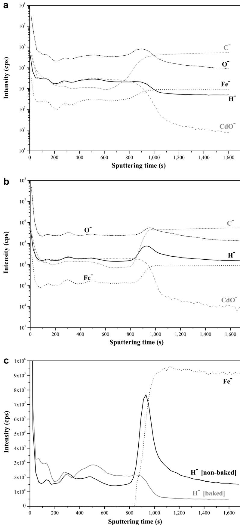
Fig. 3. Typical dynamic SIMS depth profiles measured across the Cd plating in: (a) a baked sample, (b) a non-baked sample, and (c) comparison of typical hydrogen depth profiles in baked and in non-baked samples, with the intensity being drawn on a linear scale.
