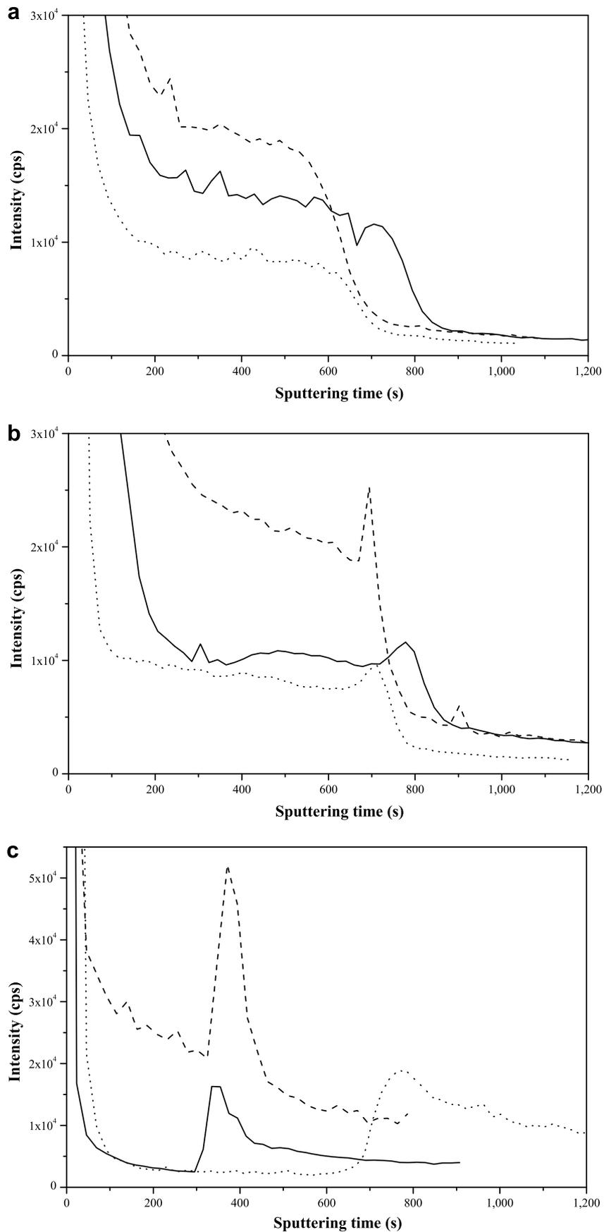
Fig. 4. Hydrogen (H<sup>-</sup>) depth profiles obtained from two baked (a–b) and one non-baked (c) samples. In each sample, the profile was acquired at three different regions.
