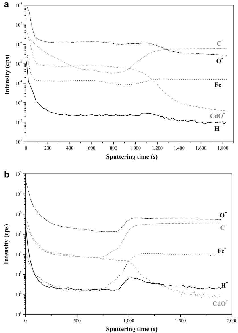
Fig. 5. Typical dynamic SIMS depth profiles measured after 16 months storage in a desiccator across the Cd plating in: (a) a baked sample and (b) a non-baked sample.
