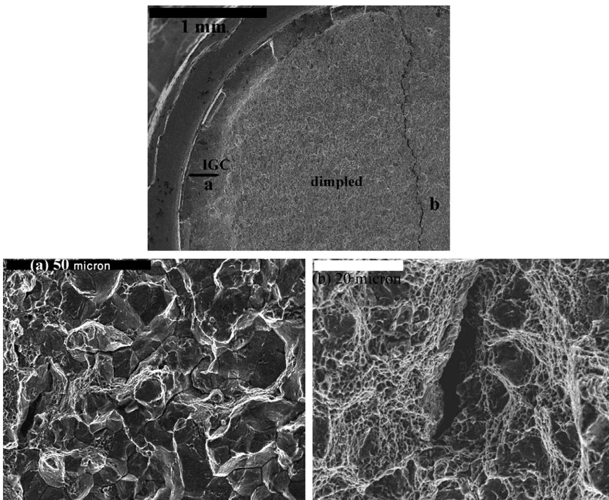
Fig. 2. SEM images of the fracture surface of a Cr-plated, non-baked TVN sample, fractured at 77% of the ultimate tensile strength. The fracture surface consists of a peripheral intergranular region (a) and an inner dimpled (overload) region (b).
