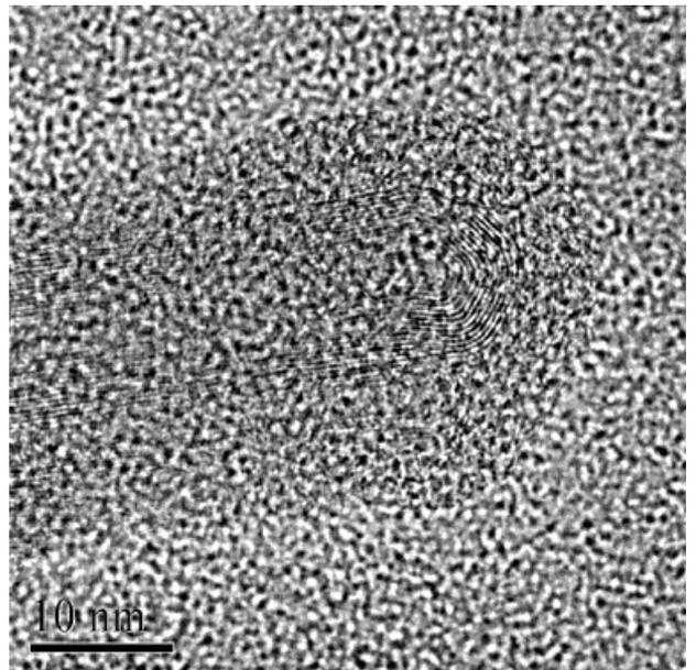
Fig. 5. Nanotubes of carbon as measured by TEM.
