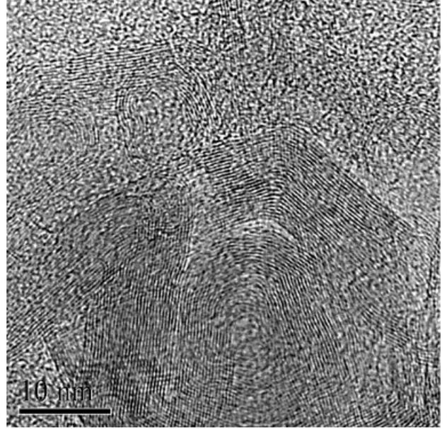
Fig. 4. Onion like carbon structures as measured by TEM.
