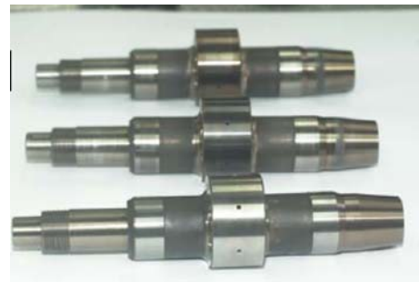
Fig. 9 The shaft with eccentric element from the first failure event (middle), a used item (top) and a new item (bottom)
