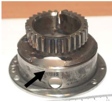
Fig. 11 Crack propagating in the gear from the first failure event
