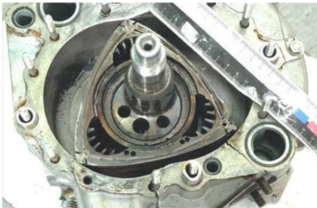
Fig. 1 A Wankel engine that failed
