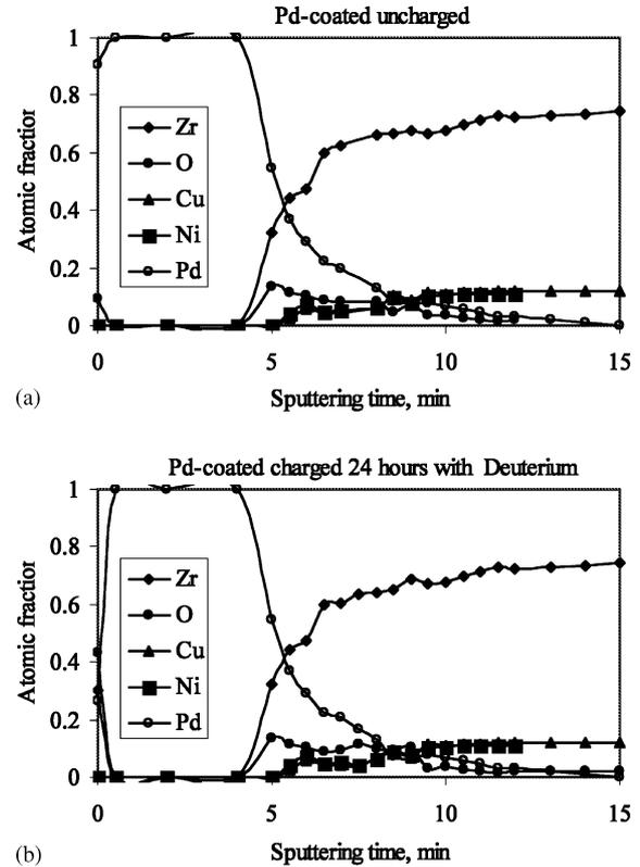
Fig. 8. AES depth profiles for (a) uncharged and (b) deuterium charged Pd-coated amorphous  $Zr_{69.5}Cu_{12}Ni_{11}Al_{7.5}$  alloy. Deuterium charging was carried out electrochemically at  $i = 5 \text{ A m}^{-2}$  for 24 h.
