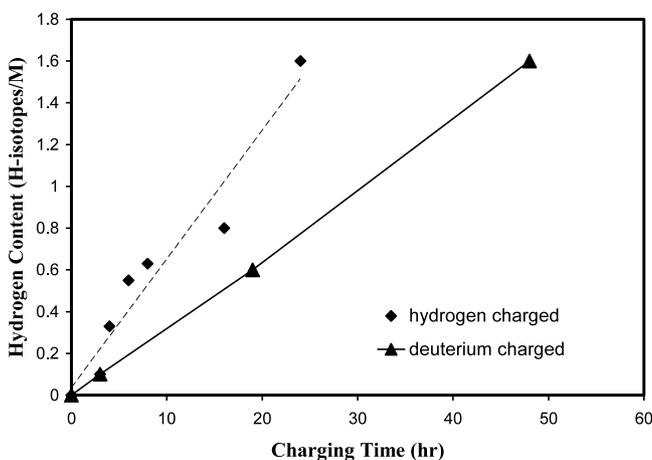
Fig. 1. Hydrogen and deuterium absorption in a Pd-coated  $\text{Zr}_{69.5}\text{Cu}_{12}\text{Ni}_{11}\text{Al}_{7.5}$  amorphous alloy, as measured by LECO hydrogen determinator following electrochemical charging at  $i = 5 \text{ A m}^{-2}$ .
