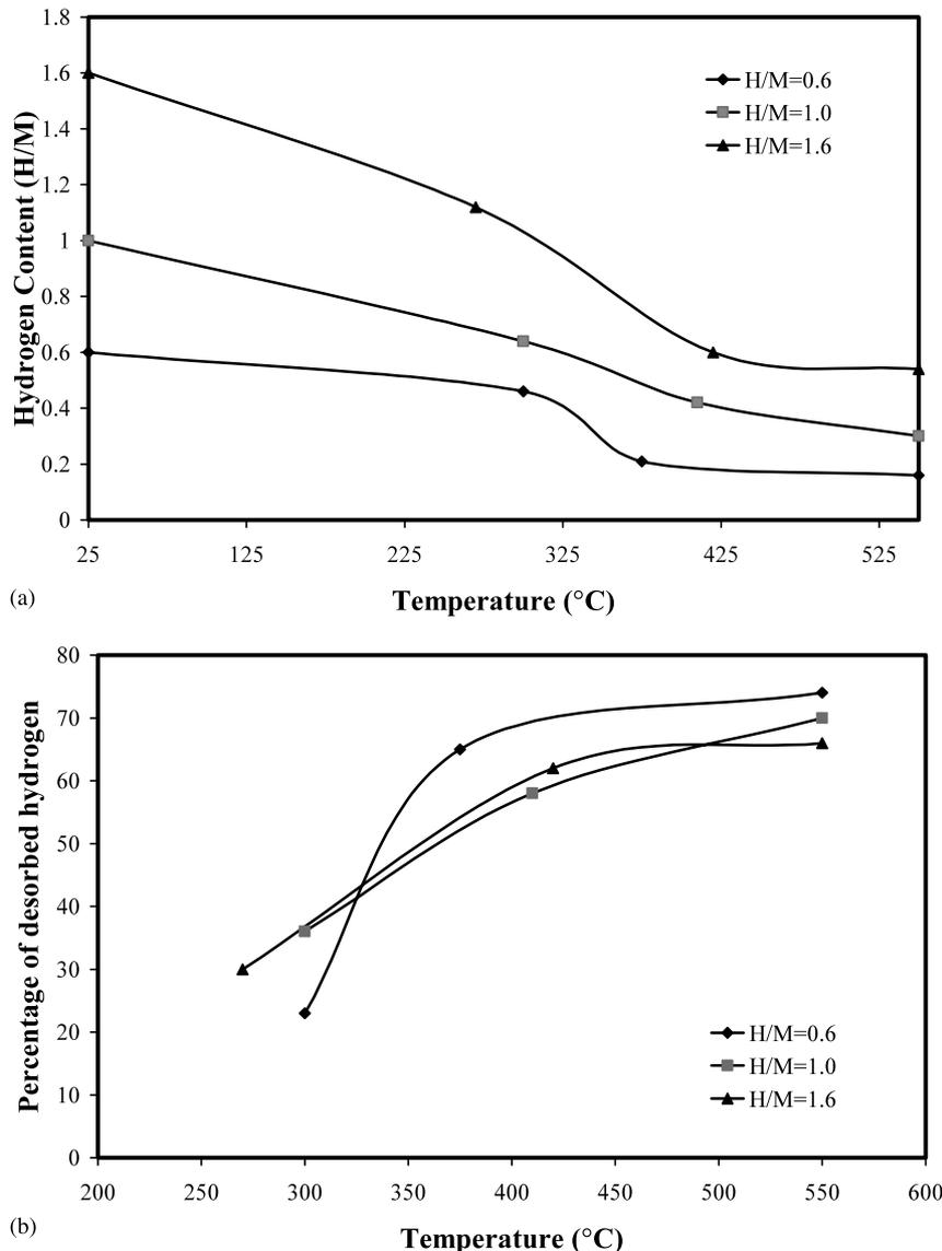
Fig. 5. Concentration of residual hydrogen (a) and percent of desorbed hydrogen (b) in hydrogen charged Pd-coated amorphous ribbons. Measurements were carried out by a LECO hydrogen determinator following DSC runs ( $\phi = 20\text{ }^{\circ}\text{C min}^{-1}$ ) to various temperatures.
