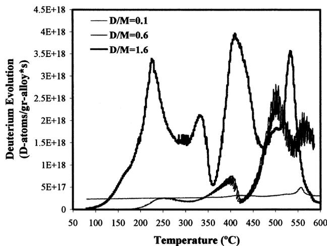
Fig. 2. TDS spectra showing deuterium evolution from Pd-coated samples pre-charged electrochemically at  $i = 5$  A m<sup>-2</sup> for different periods of time.  $\varphi = 5$  °C min<sup>-1</sup>.
