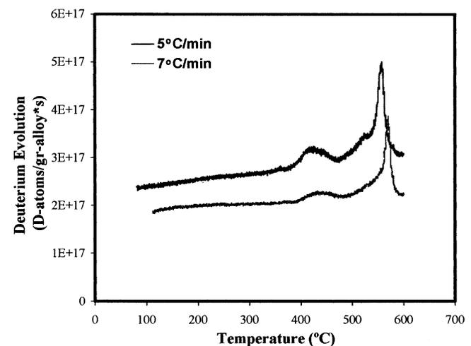
Fig. 3. Heating rate dependence of deuterium evolution from Pd-coated samples pre-charged electrochemically at  $i = 5$  A m<sup>-2</sup> to H/M = 0.1.
