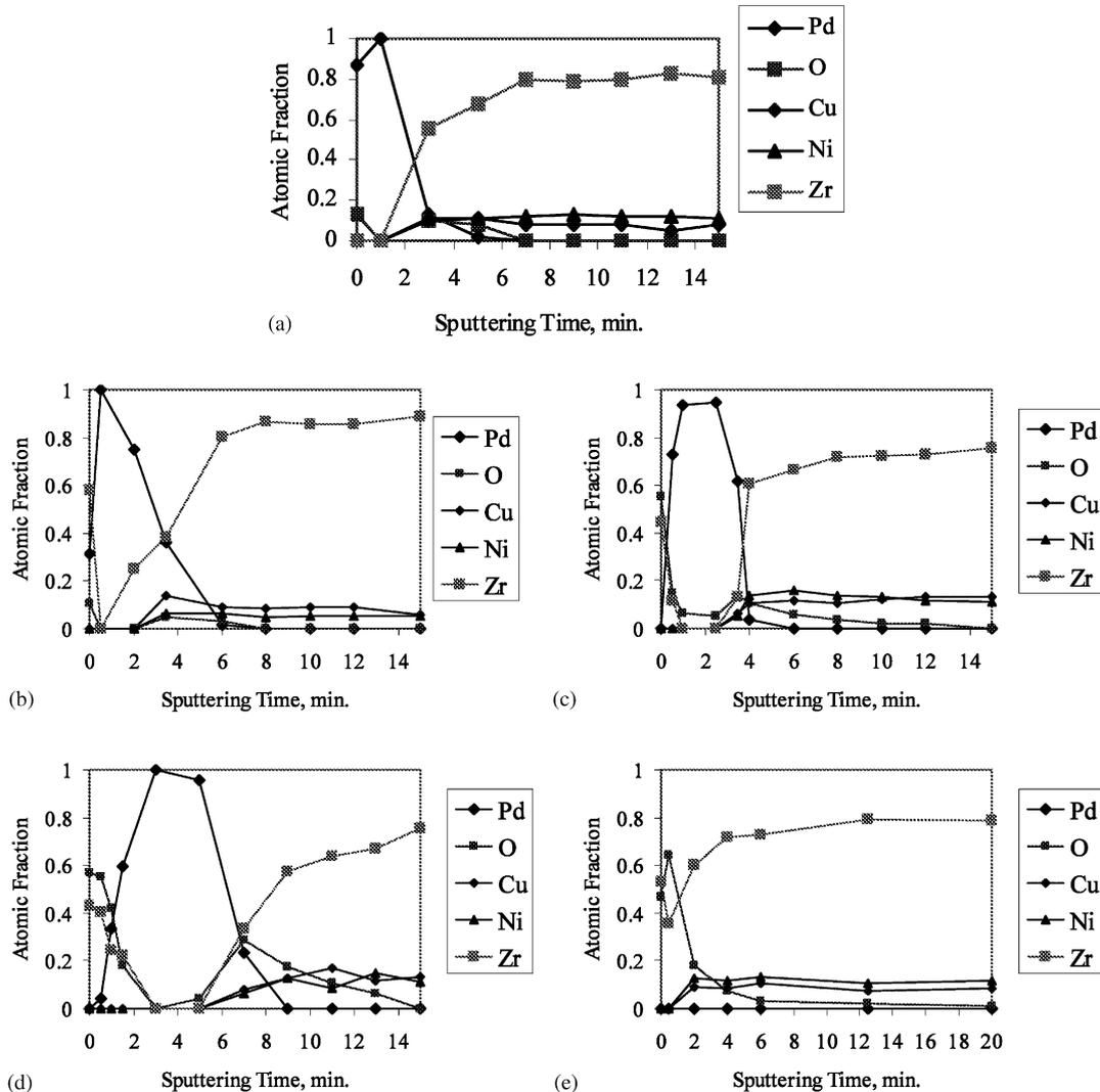
Fig. 6. AES depth profiles for uncharged (a) as well as hydrogenated (b–e) Pd-coated ribbons. Hydrogenation was carried out electrochemically at  $i = 5 \text{ A m}^{-2}$  for different periods of time, yielding  $H/M = 0.1$  (b),  $H/M = 0.3$  (c),  $H/M = 0.6$  (d) and  $H/M = 1.6$  (e).
