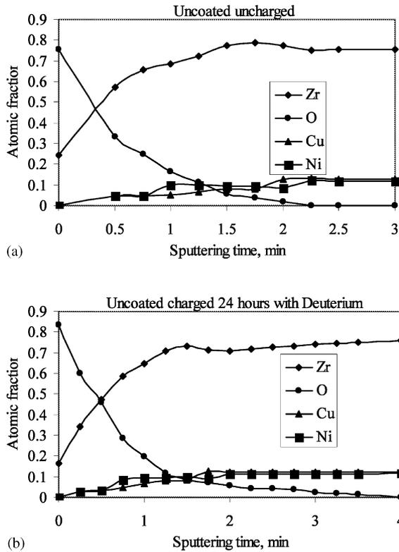
Fig. 7. AES depth profiles for (a) uncharged and (b) deuterium charged amorphous  $Zr_{69.5}Cu_{12}Ni_{11}Al_{7.5}$  alloy. Deuterium charging was carried out electrochemically at  $i = 5 \text{ A m}^{-2}$  for 24 h.
