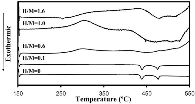
Fig. 4. DSC plots of uncharged and hydrogen charged Pd-coated amorphous samples.  $\phi = 20\text{ }^{\circ}\text{C min}^{-1}$  [6].
