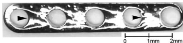
Figure 2. Hanging wire mark and oval shapes because of gas bubble flow along a heart valve frame bar made of 316LVM and electropolished via a standard DC process.
