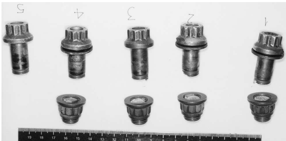
Fig. 2. Visual inspection of the failed bolts, showing transverse fracture within the threads zone.
